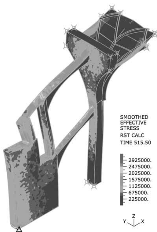
Fig. 6 Distribution of effective stress and deformation – partly supported by springs
